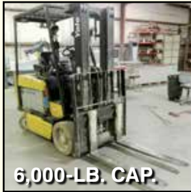
YALE Forklift Mdl. ERC0602F, 6,000-lb. cap., SS, 3-stage mast, HT, SN K502188 w/power charger, 48 volt.
