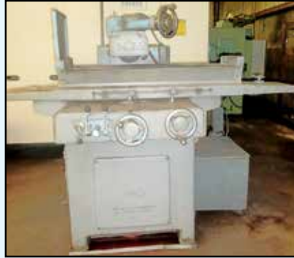
DoALL Surface Grinder , Mdl. D-8, 8" x 24" chuck, 10" x 26" travels, 12" x 3/4" x 3" wheel, SN 111.
