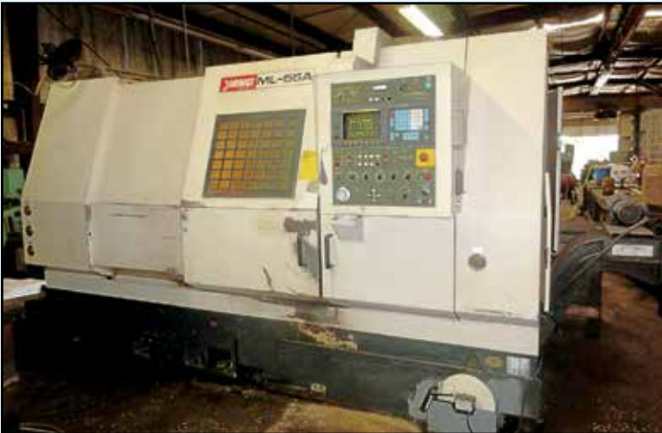
YANG Turning Center , Mdl. ML-55A, X=13.7", Z=43.3", 28.3" swing, 17.7" max. turn, 47.2" DBC, 15" 3-jaw chuck, 12-position turret, 2,000 RPM, Fanuc OT control, SN K10140.
