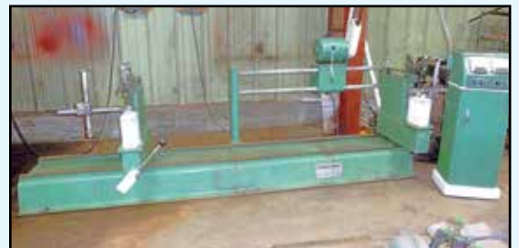
STEWART WARNER Electric Industrial Balancer , Mdl. 2380, 1,000-lb. cap., 10" cap., SN 217701.
