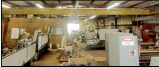
DeSHAZO Bridge Crane , 3-ton cap., w/Shaw Box 3-ton hoist, single-girder, top running, under hung hoist, pendant control.
