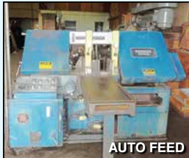
PEERLESS Automatic Horizontal Bandsaw , Mdl. HB1012, 10" x 12" cap., 1-1/4" blade, 3 HP, 0-48" feed, SN 1012A-039-79.
