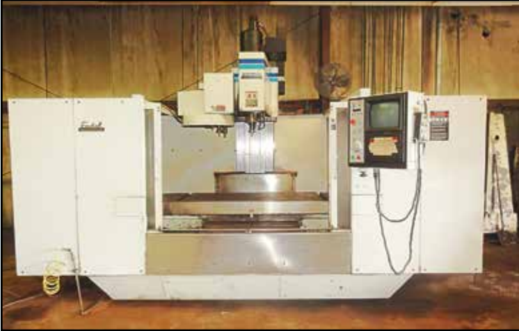
FADAL VMC6030 Machining Center , Mdl. 907-1, X=60", Y=30", Z=30", 62.5" x 30" table, 21 ATC, Cat 40, 10,000 RPM, 15/22.5 HP, CNC88HS control, SN 9609435.
