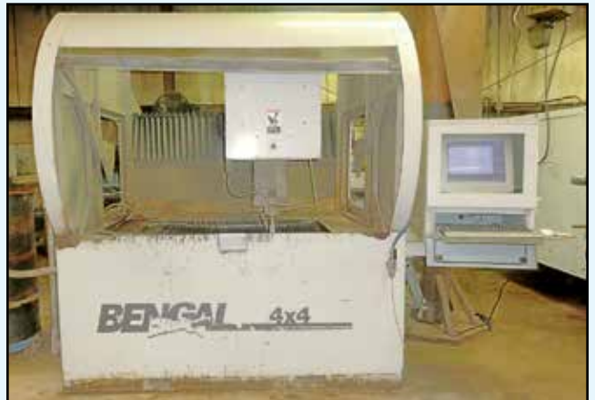
FLOW BENGAL 4x4 Waterjet , Mdl. A-00776-2, 48" x 48" x 8", Z=5.9", 50,000 PSI, flow cut control, SN 1317.
