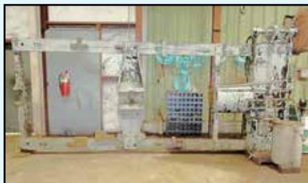
Wheel Press , 200-ton cap., 11' frame, hydraulic.
