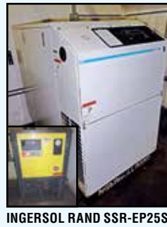
INGERSOL RAND SSR-EP25SE Air Compressor , 25 HP, 95 CFM, 125 PSIG, SN KE4096U97023.
