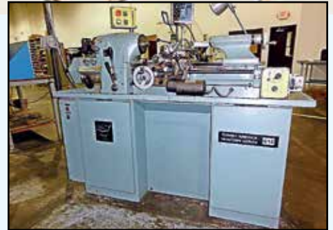
TURRET AMERICA Variturn Lathe , Mdl. 618 EM, collet closer, 1.25 HP, w/Newell 2-axis digital control, SN 8118204.
