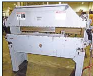
BANTAM Press Brake , Mdl. B512, 12-ton x 5', 60.25" DBH, 1-7/8" stroke, 5.75" throat, SN A9130.
