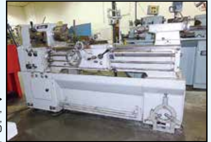
TURRET AMERICA Variturn Lathe , Mdl. 618 EM, collet closer, 1.25 HP, w/Newell 2-axis digital control, SN 8118204.
