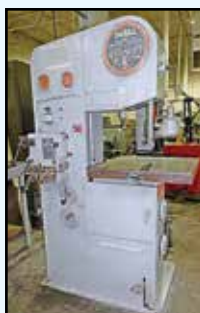
> DoALL Vertical Bandsaw , Mdl. 1613-2, 16" x 13" cut cap., 24" x 24" table, w/blade welder, SN 150-62261.
