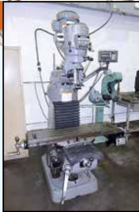
(2) BRIDGEPORT Mills , 9" x 48" table, VS, PF@X, w/Sony 2-axis DRO, SN BR275341, SN BR266815.
