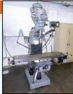
BRIDGEPORT Mill , 9" x 42" table, VS, PF@X, w/Sony 2-axis DRO, SN BR266283.
