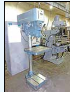
WILTON VSG Drill Press , Mdl. 2025, 20", 21" x 15" table, VS, 1.5 HP, 8-1,200 RPM, SN 153845.
