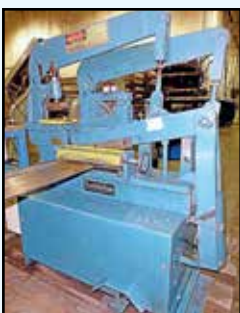
ADIRA Press Brake , Mdl. QHA-03215, 35-ton x 5' cap., 43" DBH, 4" stroke, 9.85" throat, SN 420277913, 1996.
