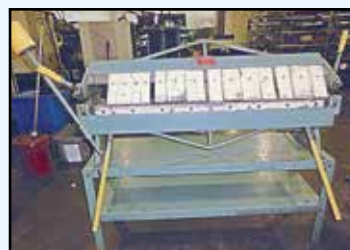
CONNECTICUT Box and Pan Brake , Mdl. U416, 4'.
