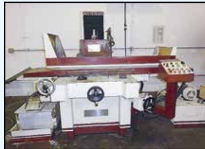
< ACER Surface Grinder , Mdl. AGS-1632AHD, 16" x 32" cap., SN 97010067, 1997.
