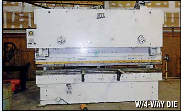
HTC Press Brake , 12' x 150-ton, 124" DBH, 2.5" RAM, 15 HP, SN N/A.
