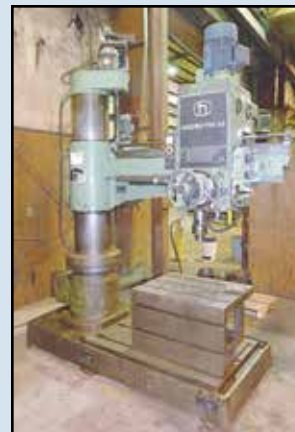
< AMERICAN Hole Wizard Radial Drill , 17' column x 6' arm, 44' x 60' box table, 30' x 20' table, #5 Morse taper, 1,200 max. RPM.
