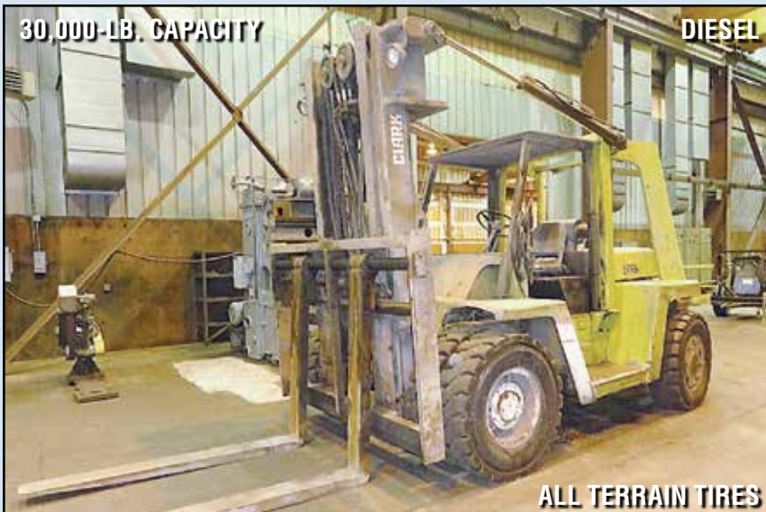
CLARK 30,000 lb. Fork Lift , dual pneumatic all terrain tires, 2-stage mast, 144" mast hgt., diesel, hydraulically adjustable forks, 9,976 hrs.
