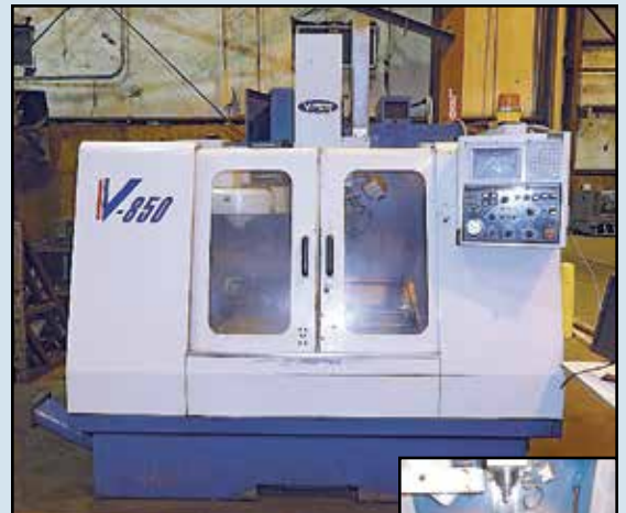
VIPER VMC , Mdl. 850-P, X=32", Y=20", Z=24.8", 32" x 18" table, Cat 40 tooling, 20-ATC, 10 HP, 8,000 RPM, w/Meldas M500 Series control, SN 912804-004, 1997.
