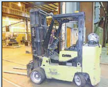
CLARK 8,000 lb. Forklift , Mdl. GCX40, LP gas, hard tires, SN GX710U-0078-9308FB, hrs. unknown.
