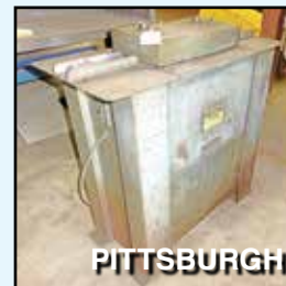
ROLL FORMER LOCKFORMER Pittsburgh Profile, 20-ga., S/N 207281.
