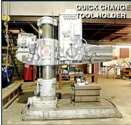
CINCINNATI Bickford Radial Arm Drill, Super Service, 11" column x 4" arm w/box table and quick change tool holder.
