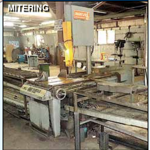
MARVEL Series 8 Bandsaw, Mdl. Mark I, 18" x 20" cap., 12' in-and-out feed, S/N 824108-W.
