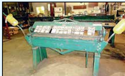
BOX & PAN BRAKE TENNSMITH Box and Pan Brake, Mdl. HB4, 12-ga., S/N 4812.
