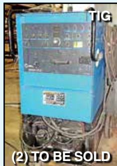
MILLER Syncrowave 250DX Welders, single-phase.
