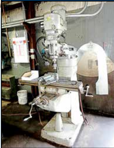
BRIDGEPORT Knee Mill, 9" x 42", variable speed, chrome hard ways, S/N 12/BR232500.
