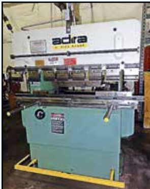
ADIRA Press Brake , Mdl. QHA-03215, 35-ton x 5' cap., 43" DBH, 4" stroke, 9.85" throat, SN 420277913, 1996.
