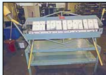
CONNECTICUT Box and Pan Brake , Mdl. U416, 4'.
