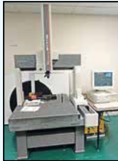
MITUTOYO CMM, Mdl. BH706, 28" x 24" x 18" cap., w/Geo Pack 500 software, SN 0421510.
