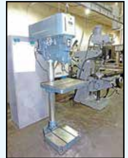
WILTON VSG Drill Press, Mdl. 2025, 20", 21" x 15" table, VS, 1.5 HP, 8-1,200 RPM, SN 153845.
