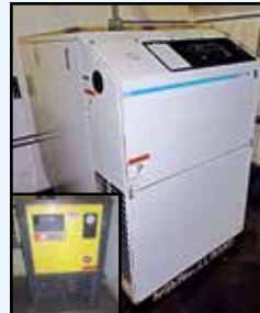
INGERSOL RAND SSR-EP25SE Air Compressor, 25 HP, 95 CFM, 125 PSIG, SN KE4096U97023.
