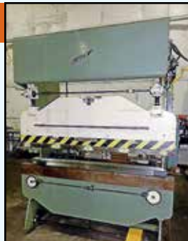
DIACRO Press Brake , Mdl. 16-72, 25-ton x 6', 5'2" DBH, 2" stroke, 9" throat, SN JE1035.
