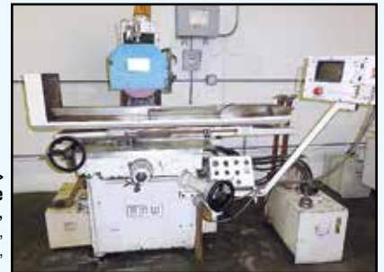
> AMW Surface Grinder , Mdl. GS-1020BH, 10" x 20" cap., SN 909236-2.
