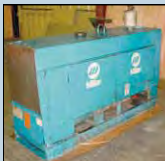
1986 MILLER 55D Trailblazer Welder/Generator , Perkins 4.154 diesel, 3 KVA, 50-450 amps, S/N JJ3209045.
