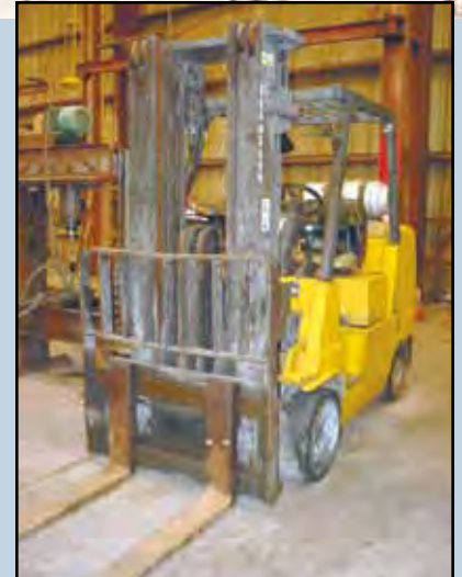
CATERPILLAR Mdl. GC45 Forklift , 10,000-lb. cap., 3-stage mast, LP gas, side shift, S/N 818701199.
